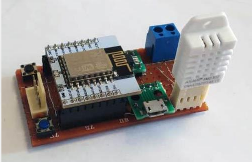
An image of a fabricated prototype of sensor nodes with ESP-12E WiFi Module, DHT11 sensor, and ACS712 sensor
